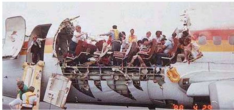
Fig. 1.3 The Aloha Airline Boeing 777 immediately after landing, April 1988.
